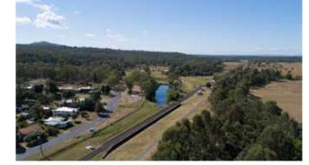
5. Grandchester The alignment has been shifted to the south to reduce severence of high value agricultural grazing/cropping land, improve the flow of water (flooding impacts) and remove the need for a high embankment through the town. A benefit of this closer-to-ground-level alignment through Grandchester is a reduction in potential noise, vibration, visual and air quality amenity impacts to residents.
