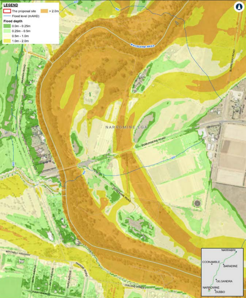
NARROMINE TO NARRABRI Existing peak depth / level (contour) - Detail - 1% AEP - Narromine Appendix H - Figure 1.1b
