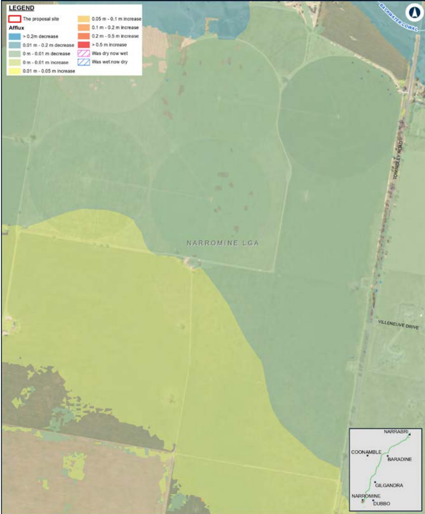
NARROMINE TO NARRABRI Change in peak flood level (afflux) - Detail - 1% AEP - Narramine Appendix H - Figure 2.1m
