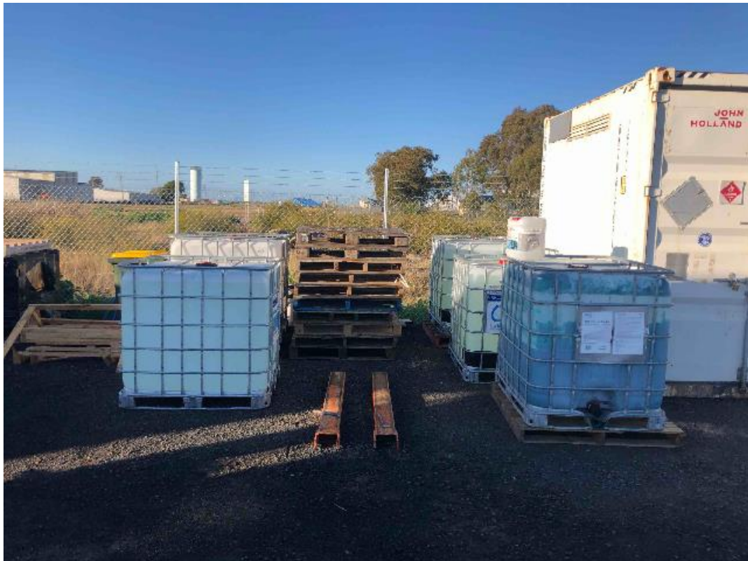
Plate 13 – PAD4 IBC's not contained in bunding
