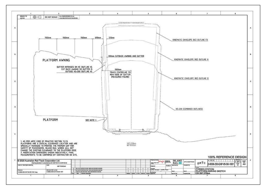
Figure 3-5: Measured schematic cross-section from platform wall through to awning and platform edges (WSP).
