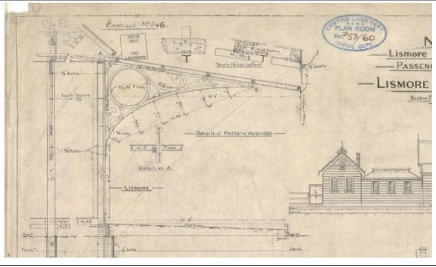
Plan of Lismore Station showing the awning overhanging the platform exactly as it does at Forbes Station.
