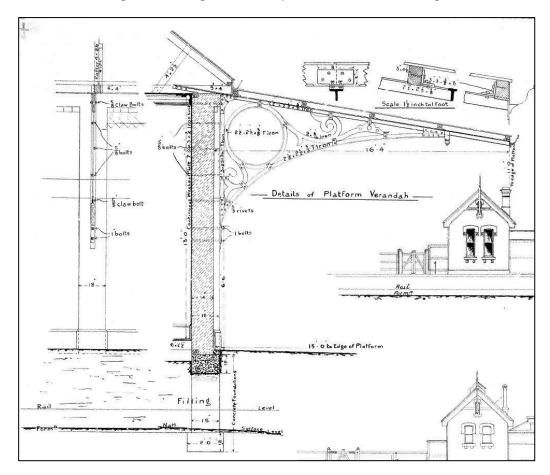
Figure 3-2: Original station plan: detail of the awning.
