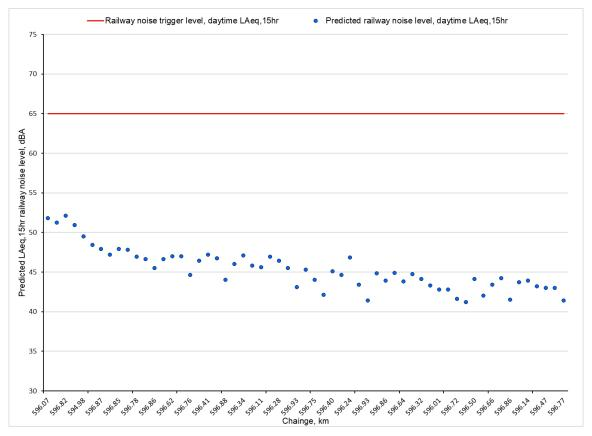
Figure C.1 Predicted daytime L<sub>Aeq,15hr</sub> railway noise levels (2020)
