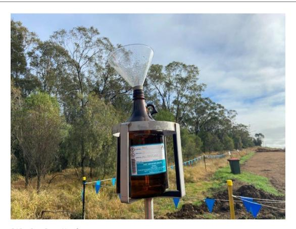
Plate 5 – PAD 6 Dust Deposition Gauge
