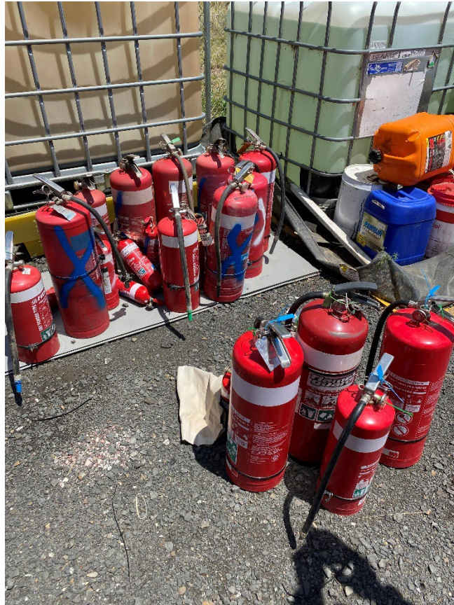
Plate 13 – Used extinguishers with collapsing bund overfilled in background at Pad 4
