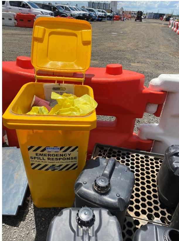
Plate 15 – Emergency spill response kit used as bin at Pad 4
