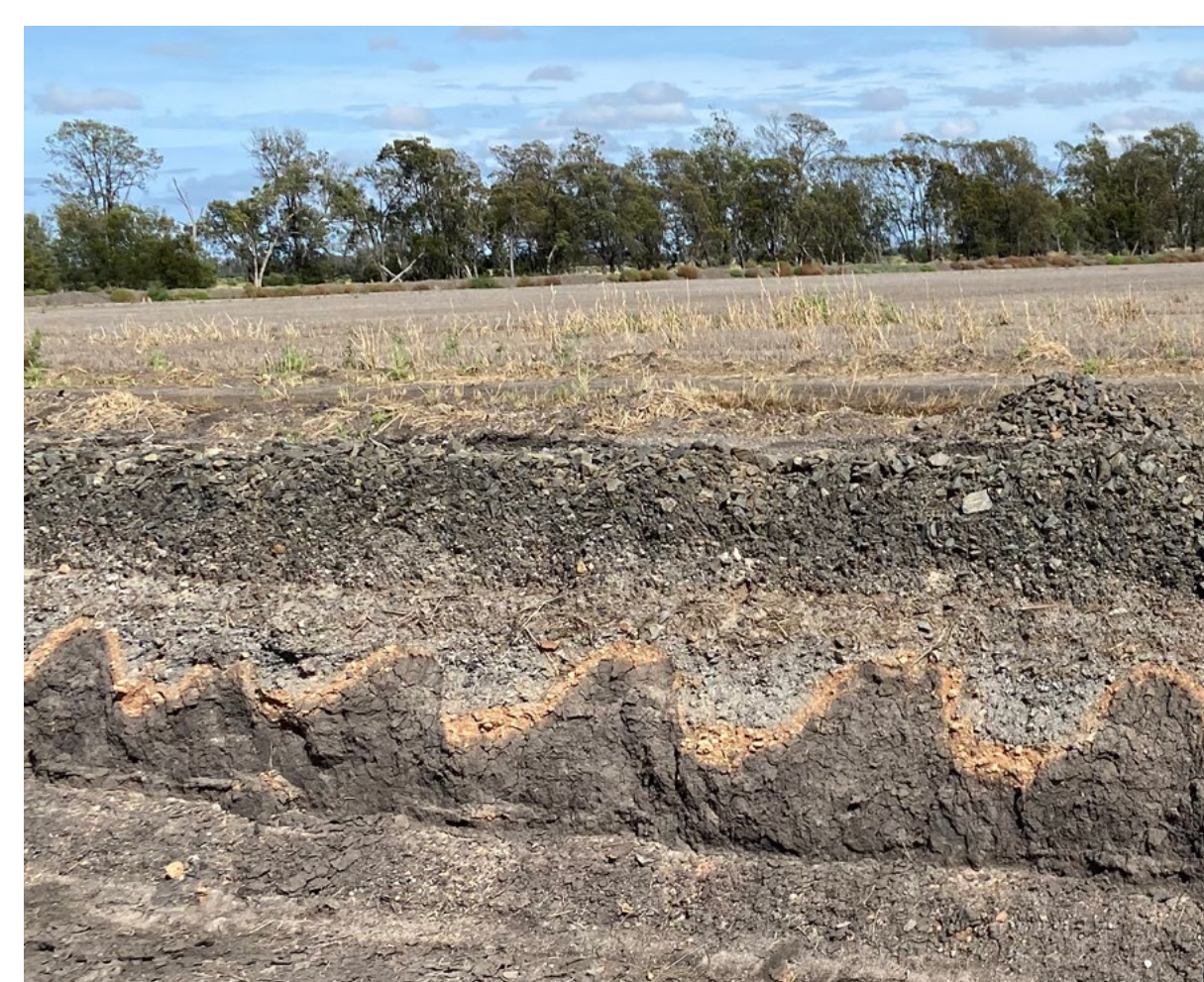
Figure 1 Left: This image presents the cumulative plastic deformation at the subgrade during the removal of the existing track. Right: image was adapted from the literature by Li and Selig (1998).
